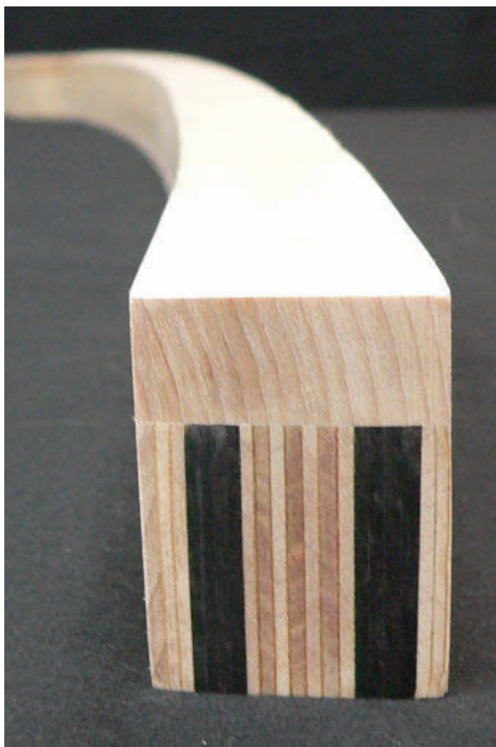
Photo 9 — The tenor bridge of instrument #22003. This bridge features vertical laminations of maple mahogany and ebony with a maple cap (note that this bridge is not yet notched!).
