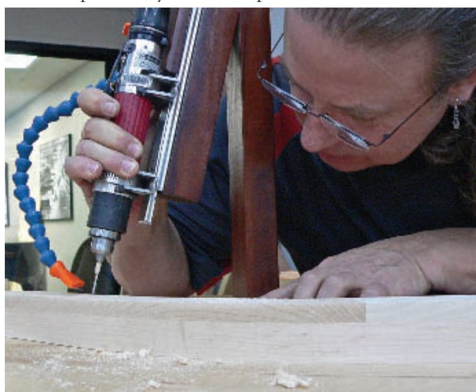
Photo 10 — Michael drilling a 220 bridge with a pneumatic drill mounted on a sliding angled drilling fixture.
