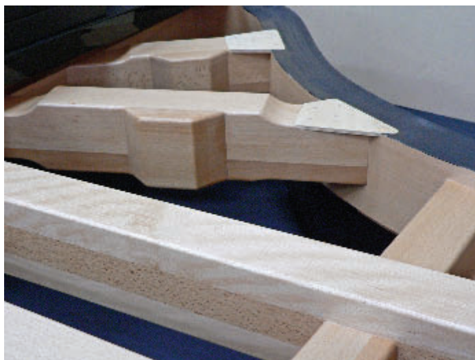
Photo 3 — Underside of the model 275 rim, showing the three-ply beech bracing.
