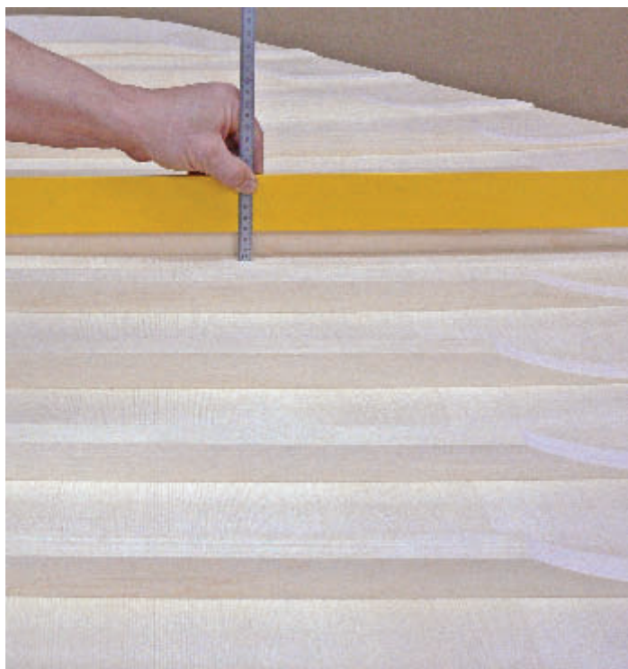
Photo 7 — The model 220 soundboards leave the press with a 22mm crown over a one meter span.
